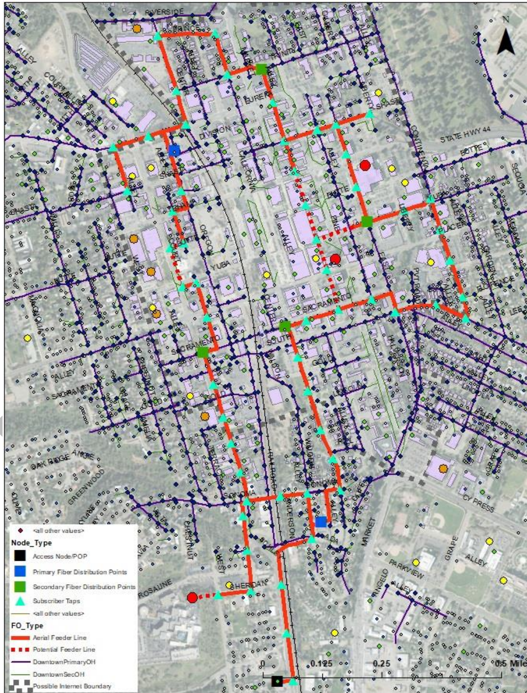
Figure 26. Fiber-optic network design for the City of Redding
