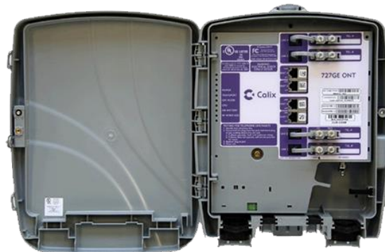
Optical Network Termination (ONT)
